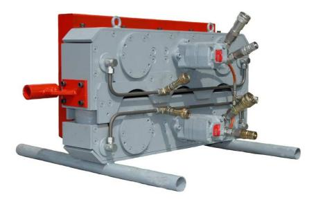
Two tubes attached to the bottom of the machine to facilitate attachment structures of the construction site with orthogonal joints.
