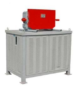
Installed power: 22 KW Pump weight: 490 Kg/pc
