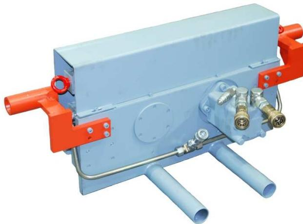
Two tubes diameter attached to the bottom of the machine to facilitate attachment structures of the construction site with joints.
