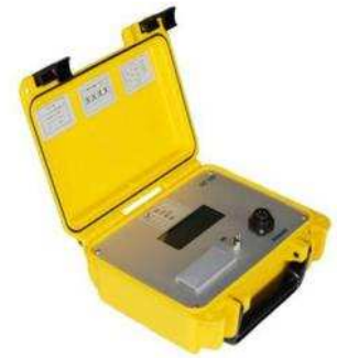
(Reading device for TTR-E-DES cells TT1000 type)
