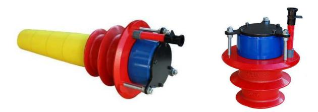
The "**D**" series active anchorage is made of the following parts: casting, preassembled D anchor plate, wedges and connection in H.D.P.E. to connect the casting to the metallic sheath. Castings have a turned plane for the plate, holes for connection to cap and formwork and a threaded grouting hole. Castings are in spheroidal cast iron EN-GJS 500-7 EN-JS-1050, which offers a high resistance to stress. Being weldable, it guarantees the maximum safety during installation.
