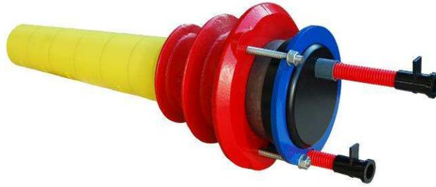
The properly mounted cap allows grouting under pressure and the total coverage of both wedges and strand protrusions from the anchorage. Qualified operators shall always be employed to carry out the installation of devices and accessories.
