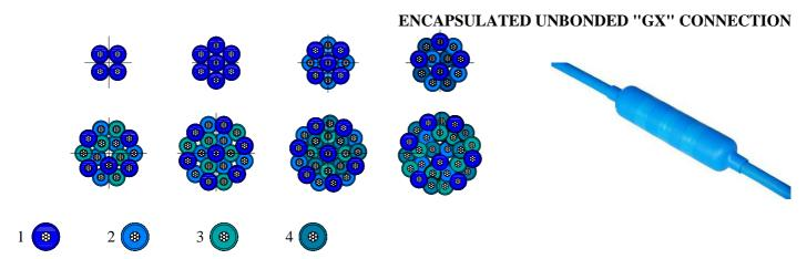
Joints "G" series were created encapsulated in the "GX" solution designed to allow single or multi stranded cables spliced in the non-adherent, while building bridges in progress, casting and shooting joints of cables. The coupling is achieved with linear monotrefolo encapsulated, with their internal pre-loaded terminals with spring-loaded device, the whole is encapsulated in polyethylene is fat.
