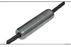
Sleeves for post-tensioning used on strand connections. Sleeve with wedges in steel 16NiCr4Pb UNI EN 10277-4.
