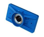
Steel plate in C40-45 UNI EN 10083/1, <u>covered in polyethylene</u> made for applications with T15, T15S and T15C strands. It is used for connecting to the pressure-closing cap.
