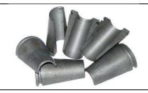
Wedges for post-tensioning on anchorages for disposable use. **16NiCr4Pb UNI EN 10277-4** steel wedges are produced in two sectors for special uses, tensioning on through cables or prelocked anchorages.
