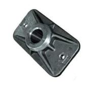
Steel plate in C40-45 UNI EN 10083/1 made for applications with T15, T15S and T15C strands, provided with thread for closing cap connection.
