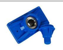
Steel plate in C40-45 UNI EN 10083/1, <u>covered in polyethylene</u> made for applications with T15, T15S and T15C strands. It is produced with thread on the edge to connect to the closing tip.
