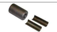
Extruded grips are made of: T15 bushes C40-45 UNI EN 10083/1, T15 shell in steel 9SMnP28 UNI 483, they are used where a compact passive anchorage is required.
