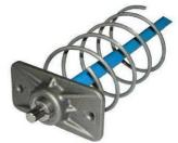
The anchorage: **active and unbonded**, "**1E15-A1**" **type.** It is supplied with a connection with the greased strand covered in polyethylene, the corrosion protection is provided by means of passivation while grouting. This application is typical for floors, diaphragms and slabs. The "**1E15-A1**" anchorage is unbonded, it may be supplied active (tensioning side) with truncated cone or rectangular pocket former to connect to the formwork.
