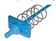
The anchorage: **passive**, **unbonded and encapsulated**, "**1EX15-D2**" **type**. It is made with the total encapsulation of the polyethylene covered anchorage, with the greased strand covered in polyethylene. The "**1EX15-D2**" anchorage is unbonded, it is supplied passive, factory prelocked or to lock on site by using a **B300KN jack**. This application is typical of industrial floors, foundation piles, diaphragms and slabs in a highly corrosive environment for the whole system.
