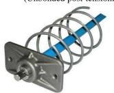
The anchorage: **passive, unbonded, "1E15-D1" type.** It is supplied with a connection with the greased strand covered in polyethylene. This application is typical of industrial floors, diaphragms and slabs. The "1E15-D1" anchorage is unbonded, it is supplied passive, factory prelocked or to lock on site by using a **B300KN** jack. It is directly covered while grouting and its corrosion protection is obtained by means of passivation while grouting.
